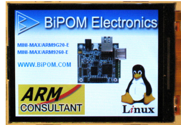
MINI-MAX/ARM9260-E Ethernet, 2 USB ports, ATMEL AT91SAM9260
